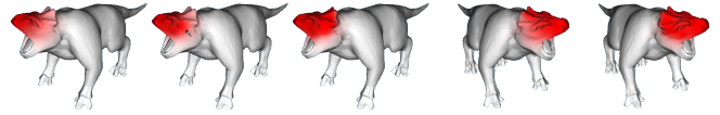
Fig. 16. Just like painting texture colors, an animator can now 3D paint high-resolution skinning weights and see their effect immediately. In this example the weights for the bony skull of the animal are painted to make it move rigidly with the rest of the head. Please see the supplemental materials for a video of this example.
